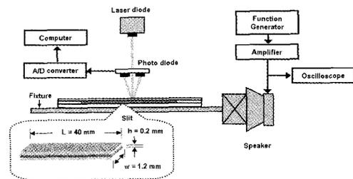
Fig. 1 Schematic diagram of the light-reflection aggregometer with vibrating mechanism
