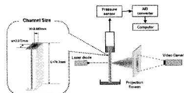
Fig.1 Schematic diagram of the laser-diffraction slit-rheometer (LDSR)
