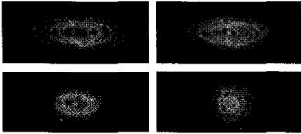
Fig. 2 Laser diffraction patterns at various shear stresses (a)  $\tau_w=31$  Pa, (b)  $\tau_w=12$  Pa, (c)  $\tau_w=3$  Pa, and (d)  $\tau_w=0$  Pa.
