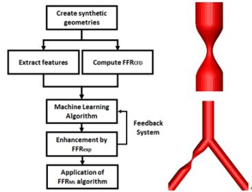
Fig. 1 (Left) Overall flowchart of ML FFR development process. (Right) Two types of base synthetic model (Straight type and Vifurcation type).
