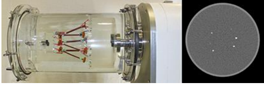
Fig. 26 Motion phantom experiment (left) and an axial slice (right)
